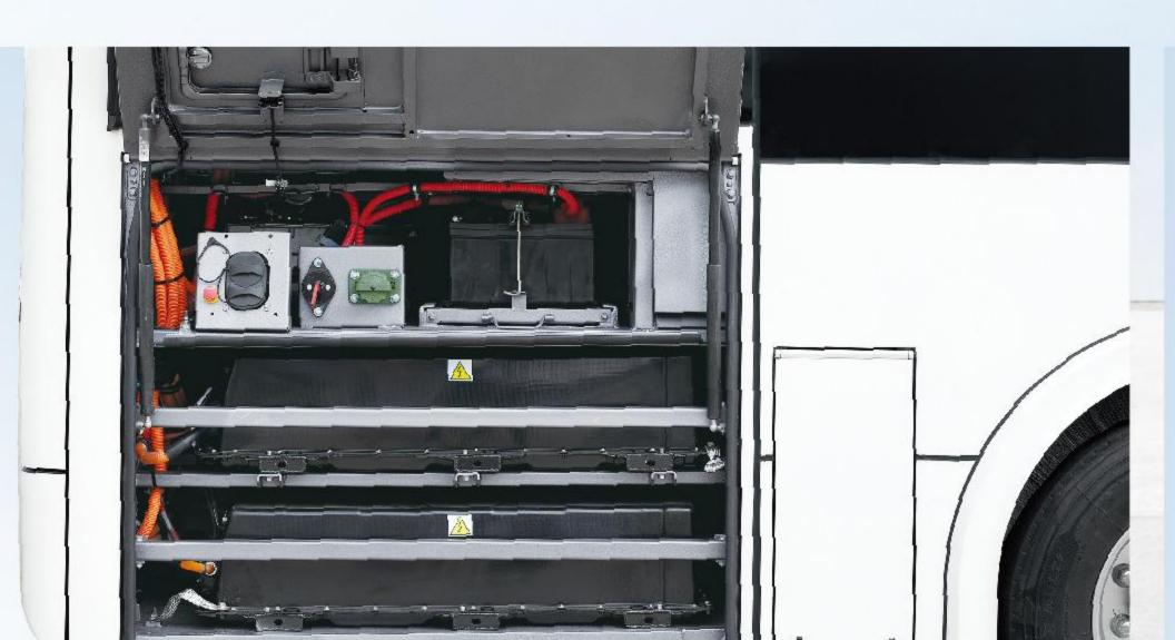
Pull-out design for low voltage battery rack
