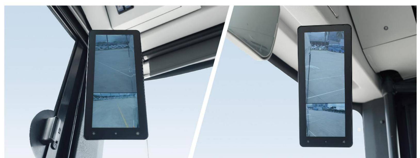
Equipped with ERM Electronic Rearview Mirror, there is no blind spot in the field of vision, and there is no obstacle to driving on rainy days and at night.
