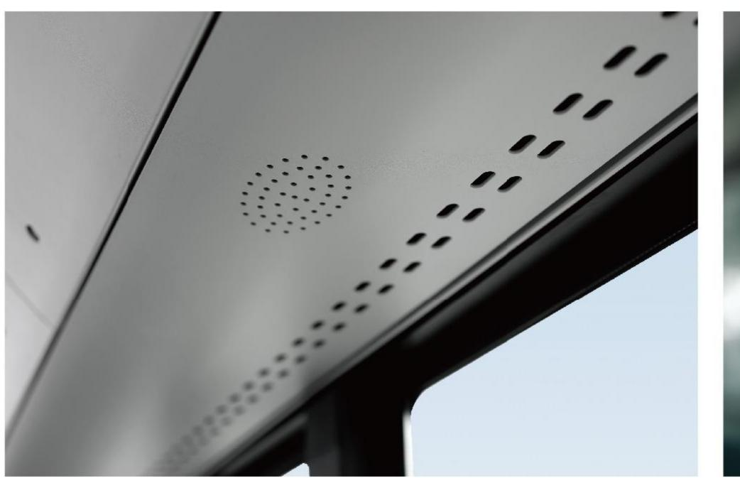
Direct cascade cooling with finer and more uniform airflow for better cooling
