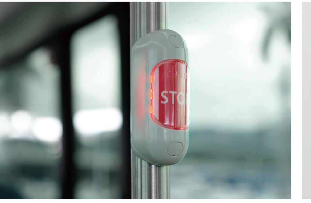
Large stop button, backlit display, more convenient to use Equipped with USB,convenient for passengers to charge
