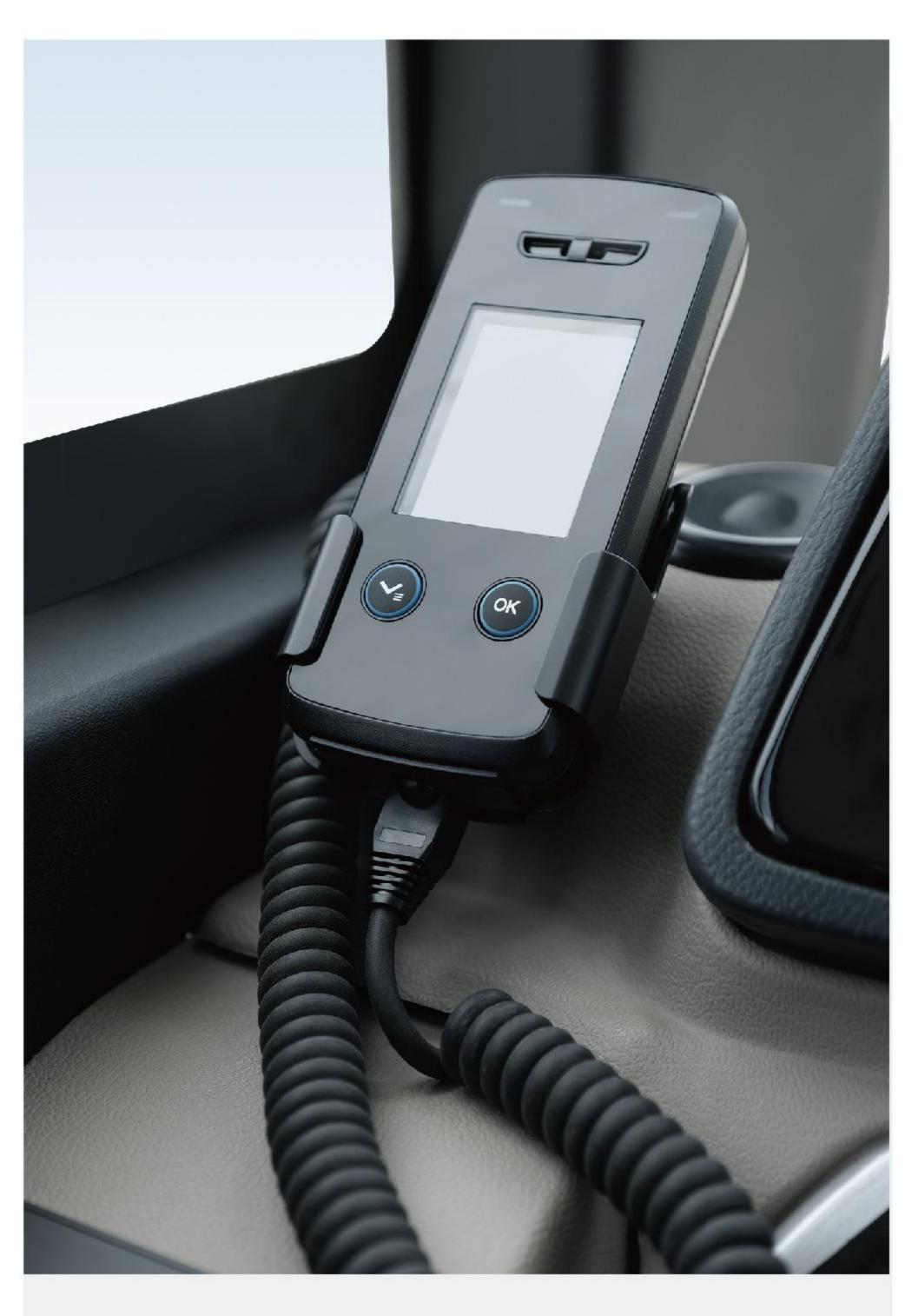
Equipped with Drager alcohol lock to prevent drunk driving.
